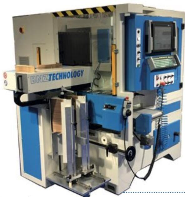
Additionally, the TWISTER machines are equipped with numerical control and digital motors.
