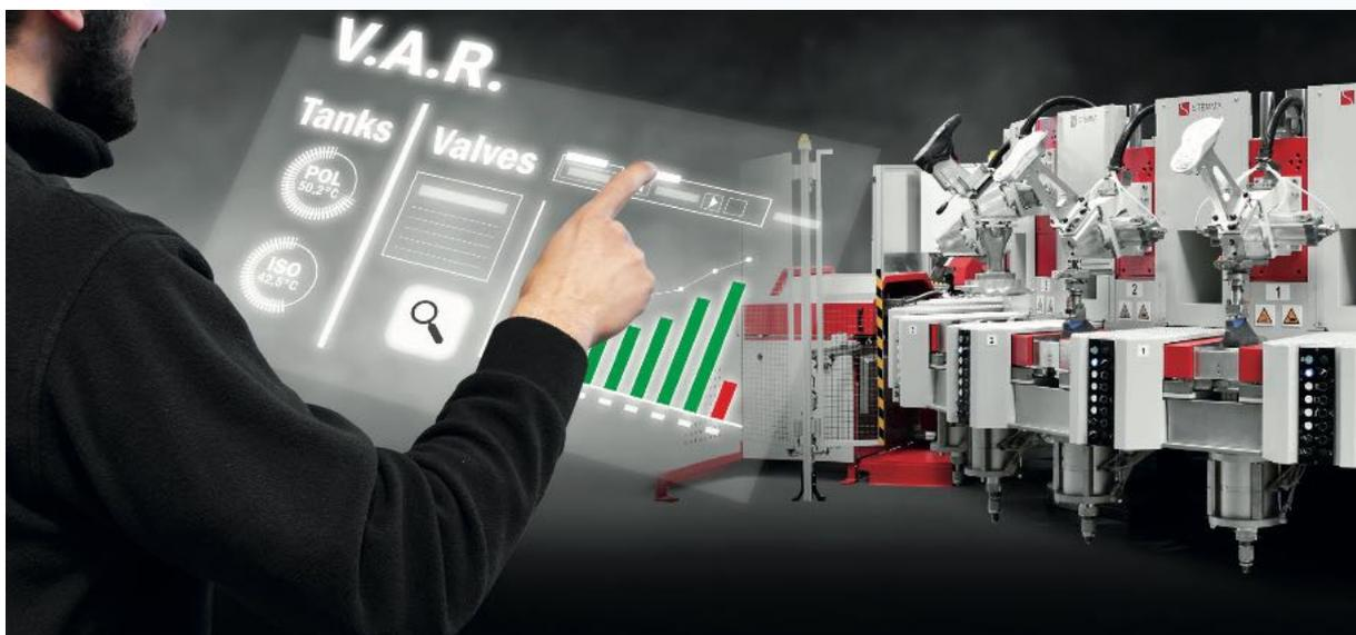
► Polyurethane direct-injection machines are among the most advanced technologies for footwear production available on the market. These machines are extremely efficient and suitable for manufacturing a wide range of shoes, however, being particularly complex, they must be attended by expert engineers for both working parameter setting and troubleshooting, in case issues arise during production. Very often, though, only a few engineers possess the information and knowledge required to
