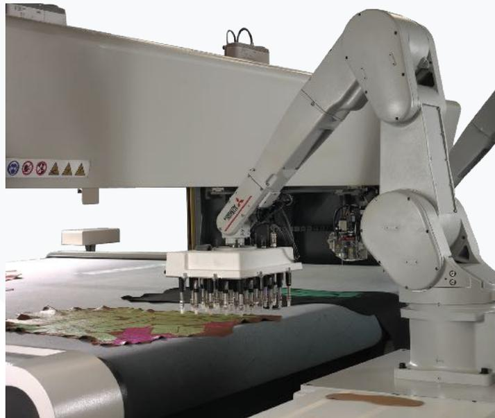
equipped with an innovative, specially designed gripper. The gripper uses a matrix of 30 suction cups, each independently controlled, driven by a special software that determines how many and which suction cups must be activated in relation to the piece geometry and position in the cutting layout, where the robot must position itself, and how it must
